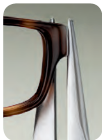
Parallel closing jaws grip frame securely
