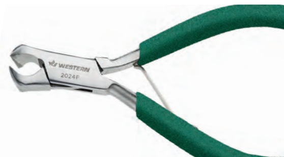
▲ Oblique Head End Cutting Plier Ref: 2024F This heavy-duty cutting plier has a 24mm long cutting edge. The head tapers to a fine point to cut screws flush in restricted areas. Use only on soft metals and plastics.
