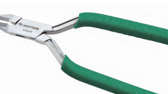
▲ Concorde Tungsten Carbide Side Cutting Plier Ref: 5026F These 'top of the line' cutters combine tungsten carbide steel cutting tips with military grade superior tensile-strength stainless steel. Comfortable foam covered extra leverage handles provide precise control for nearly flush cuts. 13mm wide cutting edge and 6-1/2" long.
