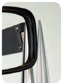
Non-parallel jaws can damage thick frames
